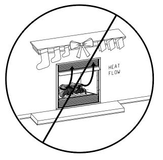
No greeting card, stockings or ornamentation of any type should be placed on or attached to the fireplace. This is a heating appliance. The flow of heat can ignite combustibles.
